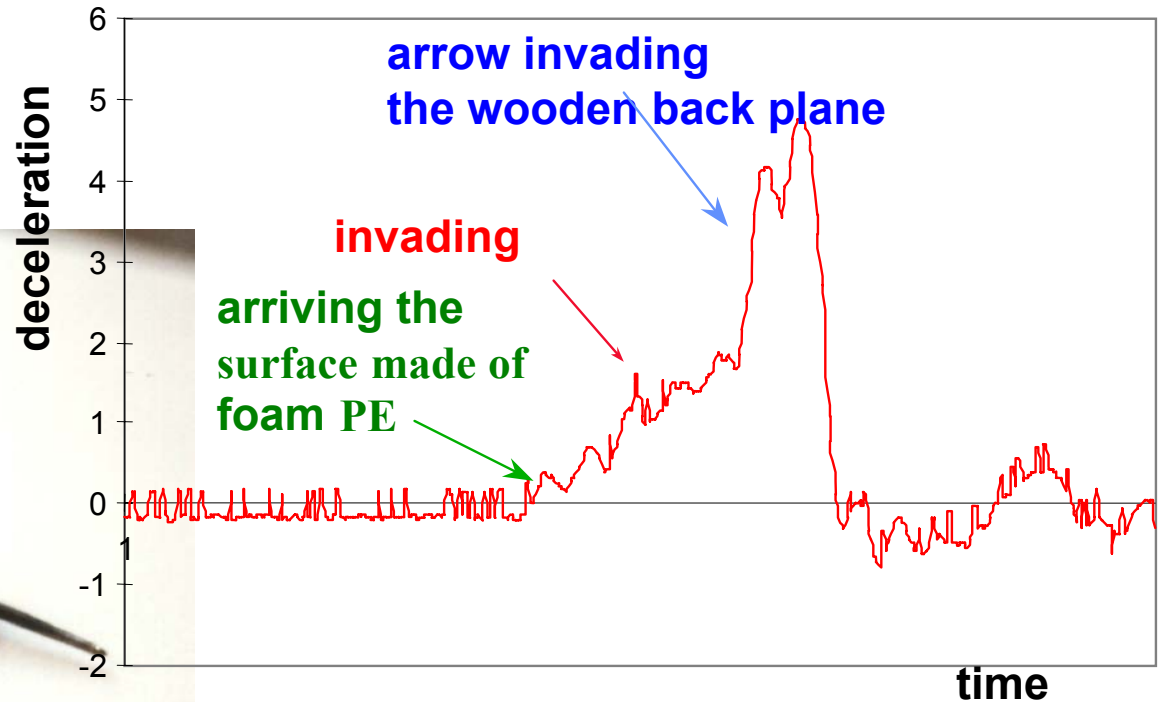
Passive SAW sensor fixed to a dDart arrow, invading the target
