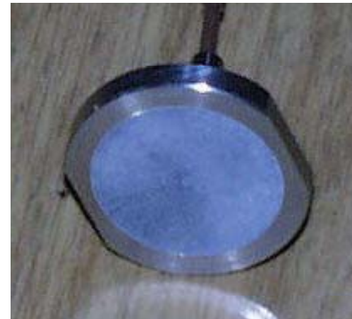
Antenna in a steel package filled with polymer (diameter = 20mm).
