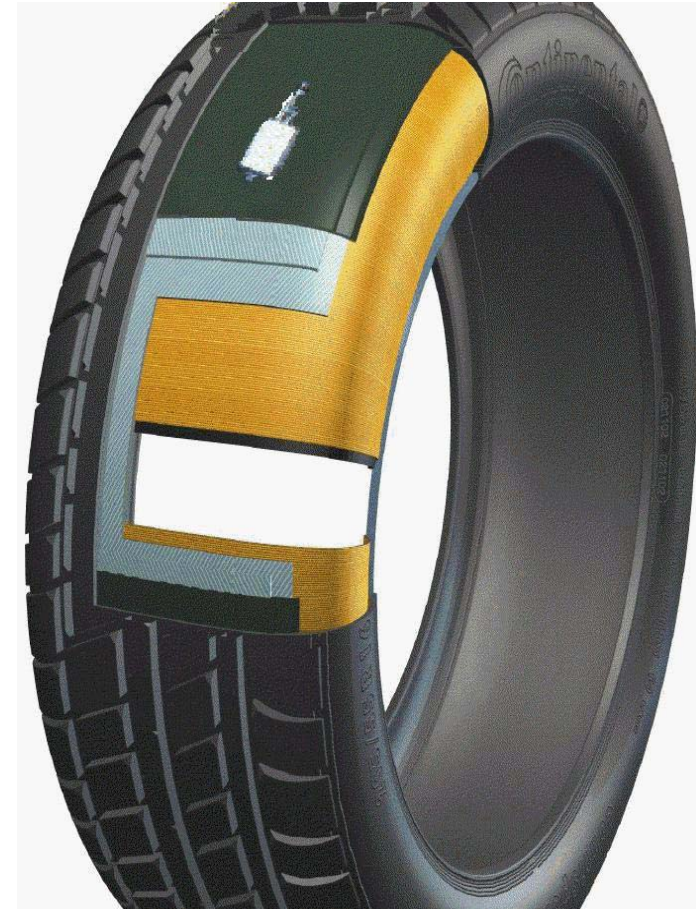
SAW sensor integrated into a standard tire
