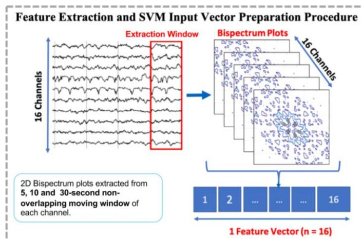
Figure 2. Feature Extraction Procedure Using Bispectrum Analysis.
