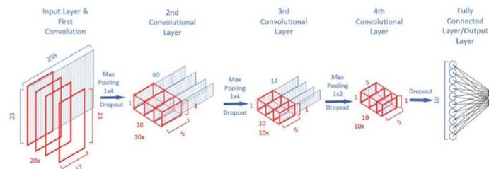
Fig.: CNN architecture for RISC-V based hardware implementation for future implantable system
